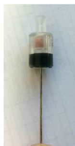
Cartridge after elution of trapped drugs from raw blood
