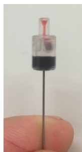
250μL raw blood tapped on μSPEed cartridge
