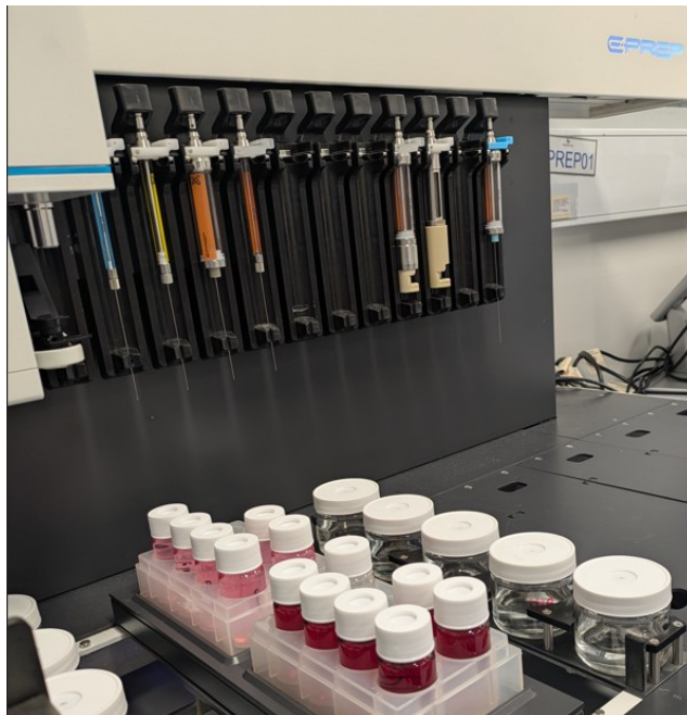
Figure 1: Automated Extraction of Vitamin B12 Identification and Assay using ePrep ONE
